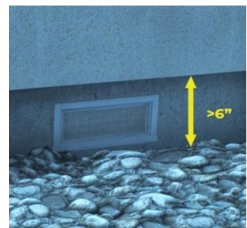
Embers accumulate against homes at the base of exterior walls and on other horizontal surfaces like decks that can ignite the home.
