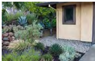
Firesafe vegetation setback 5 feet with gravel path
